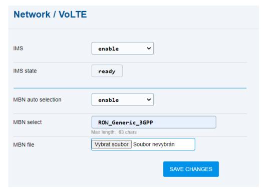
Turn on the IMS function on the Network / VolTE card to enable the VolTE function in the device. Data is enabled by the device by default, use the Network / WWAN card to change the setting. Make sure that the Network technology value on the WWAN card is always LTE (i.e. connection to LTE network) for the VolTE calls.
