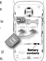
"G&W" (on the right hand side in the drawing) supports UMTS/GSM (3G) and the card slot marked with "GSM" (on the left hand side in the drawing) is limited to GSM (2G) only. When using only one SIM card, in order to use all the phone's services via 3G networks you must place the SIM card in card slot "G&W".
