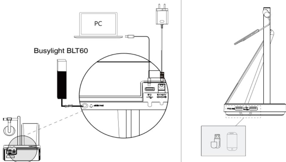
**Note:** Please make sure you connect the base to a DC power supply, not just the USB power supply. The included USB-A to USB-C cable cannot be used to connect other devices (for example, mobile device) to the USB hub port.
