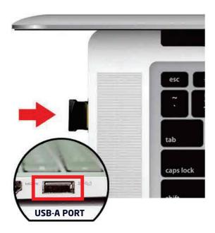
**1.** Plug the USB connection on the Bluetooth Dongle into your PC, Mac or device.
