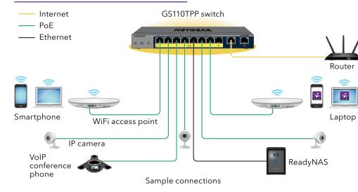
1. Connect devices to the RJ-45 PoE+ network ports on the switch front panel. Use Category 5e (Cat 5e) Ethernet cables terminated with RJ-45 connectors to make Gigabit connections.
