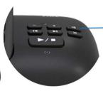
Press and HOLD the registration button on the base station for 4 seconds until you hear a beep/tone
