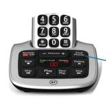
Press and hold Phone on the base until you hear a beep and the In use light starts to flash.
