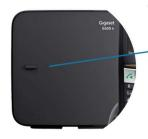
Press and HOLD the registration button on the base station for 4 seconds until you hear a beep/tone
