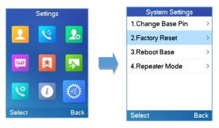
Figure 37: Resetting the Base Station
