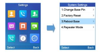
Figure 36: Rebooting the Base Station
