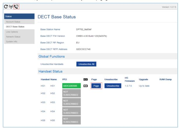
Figure 15: Locate Handsets via Web UI
