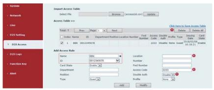
**Note**: If the RFID/IC card read data is reverse order, you need to "EGS settings" in the "Card Reader HF Card Data Reverse" open.
