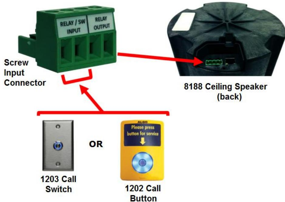
**1202 Call Button:** A pair of wires from the terminal block on the back of the 8188 can connect to the **centre pair** of the modular connector at the back of the Call Button.
