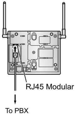
5. Install the CS temporarily for the site survey. Install the CS at least 2 m above the floor, and place the antennas so that they are pointing in directions that are 90 degrees apart (for antenna diversity), as follows:
