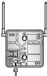
3. Switch all DIP switches on the CS from ON to OFF.
