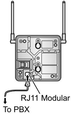
2. Pass the cable through the groove of the CS (in any direction depending on your preference).
