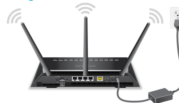
Connect the modem router to a power source.
