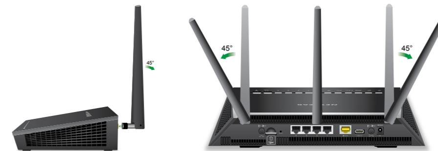
Attach and tighten the antennas on the threaded antenna posts.
