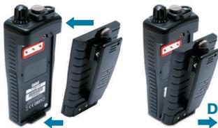
1. To attach, locate the pegs on the bottom of the battery into the slots on the radio and press the top of the battery against the radio. Secure battery by tightening the screw clockwise by hand. (Do not use any implement or over tighten) (C).
