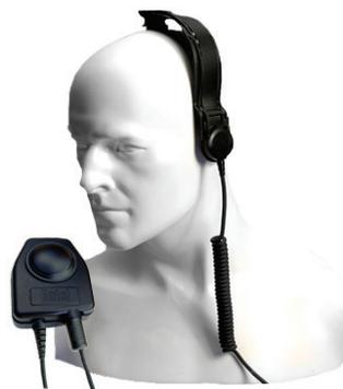
The CXR5 incorporates a high performance, low profile, bone conductive skull microphone that provides clear audio transmission even in the noisiest of environments. Unlike conventional headsets, the bone conductive skull mic is not adversely affected by external sounds. The incorporated high quality earpiece ensures loud and clear reception.
