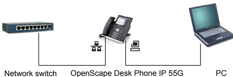
Using this connection option saves one network port for each switch used and requires fewer or shorter network cables when arranged correctly.
