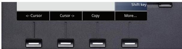
You operate the display editor using the softkeys (→ Page 23), the keypad (→ Page 26) and the navigation block (→ Page 22):
