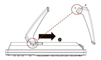
A to A gives a 50 degree tilt B to A gives a 30 degree tilt
