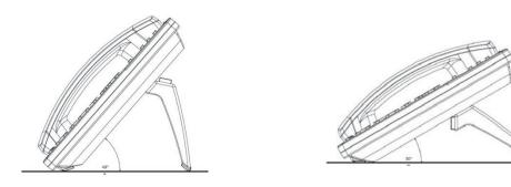
To attach the stand to the phone you will see 2 sets of slots on the rear of the telephone base and 2 sets of notches on the top of the stand ( marked A & B in the diagram beow) . For illustration purposes we are using the 50 degree angle set up.
