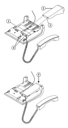
Figure 6. Installation of Bay Option Modules
