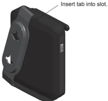
4. Check to make sure the plate is secure at top and bottom. It should be flush with the base station body.
