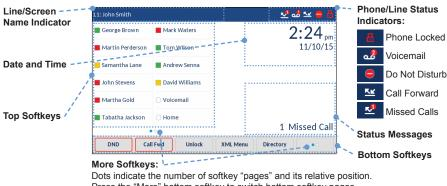
Press the "More" bottom softkey to switch bottom softkey pages Swipe left and right in the top softkey area to switch top softkey pages.
