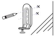
2. Remove the wall mounting bracket and check the reception strength of the Baby unit and camera angle before drilling two holes in the wall using a 5mm drill hit
