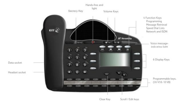
This diagram illustrates the V16 phone which has 16 programmable keys.
