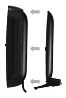
Place the cover in the notches on the back of the base station and click into place (not if mounting on the wall).
