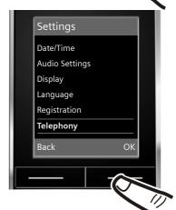
Press down on the control key until the Telephony menu appears on the display.
