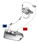
Figure 30: Connecting using an electronic-hookswitch adapter (Jabra LINK series)
