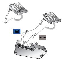
Figure 12: Connecting to a desk phone without a headset port
