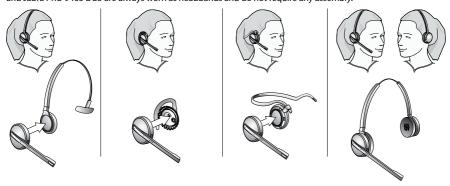
Figure 10: Assembling and wearing the Jabra PRO headset in various styles
