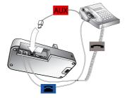
Figure 19: Connecting to a GN1000 Remote Handset Lifter
