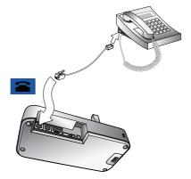
Figure 13: Connecting to a desk phone with a headset port
