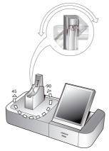
Figure 8: Adjusting the headset cradle angle on the base
