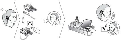
Figure 17: Setting the microphone level manually
