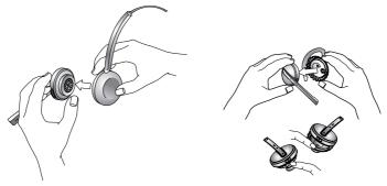
Figure 45: Detaching a wearing-style attachment from the headset
