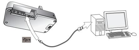
Figure 31: Connecting to a computer
