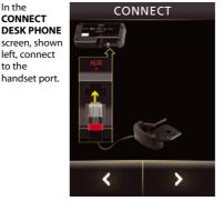
screen, shown left, connect the control cable attached to the GN1000 to the base's AUX port.
