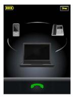
Figure 36: A disconnected target phone is shown greyed out on the touchscreen
