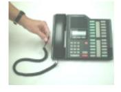
**Step 2.** Plug the handset coiled cord that you just removed into the OFFICE KONNECTOR connector jack labeled **HAND SET**.
