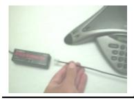
**Step 5.** Connect the power cord into the OFFICE KONNECTOR then plug the AC adapter into an AC wall outlet (unit will not operate without a power supply).
