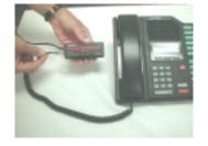
**Step 3.** Plug the short cord on the OFFICE KONNECTOR into the handset jack on the telephone base unit (desk set).
