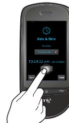
9 Adjust the date or time using + or -. Press **OK** to confirm.
