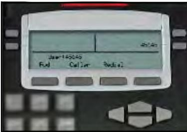
**Figure 10: Logged on to an Avaya 2033 IP Conference Phone using an IP Phone 2004**
