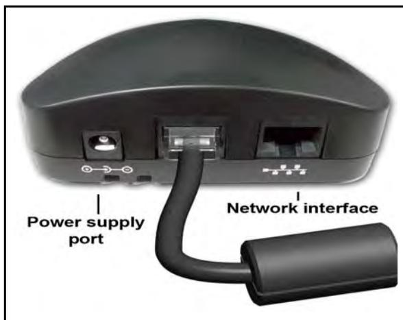
2. Connect the CAT5 Ethernet cable attached to the PoE module to the IP Phone. Thread the CAT5 Ethernet cable through the channel on the bottom of the IP Phone and plug it into the PoE module port on the IP Phone.
