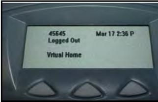
When activated for Virtual Office by a remote telephone, your office telephone is *logged out* and is no longer operational.
