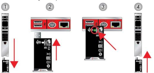
Figure 1: Recharge the Battery: RealPresence Group 300, 310, 500 and 700 Systems
