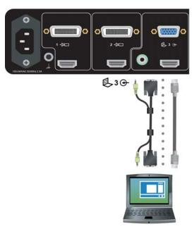
Figure 2: Connections for a RealPresence Group 700 system
