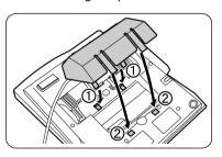
4 Pull down the handset hook until it locks, so the tab holds the handset.
