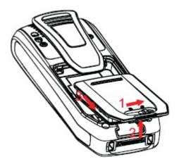
Figure 14: Easy Replaceable Battery - Unlock the Lid and Remove the Battery
