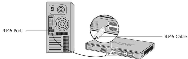
Figure 4-1 Connecting the RJ45 Port
