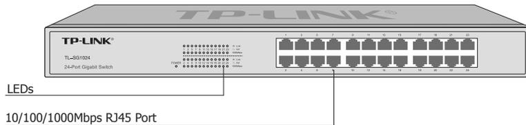
Figure 1-2 Front Panel of TL-SG1024
