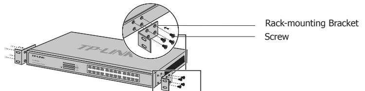
Figure 2-2 Bracket Installation
