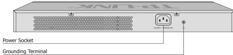
Figure 1-8 Rear Panel of TL-SG1024/TL-SG1016
