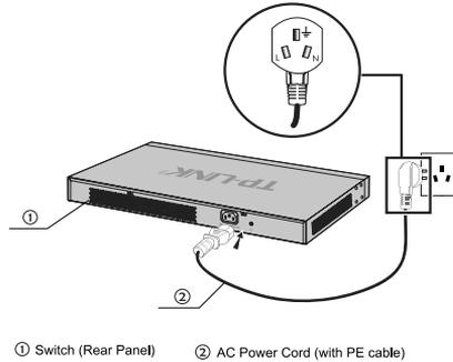
Figure 3-2 Connecting to the Ground
