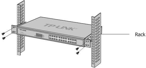
Figure 2-3 Rack Installation
