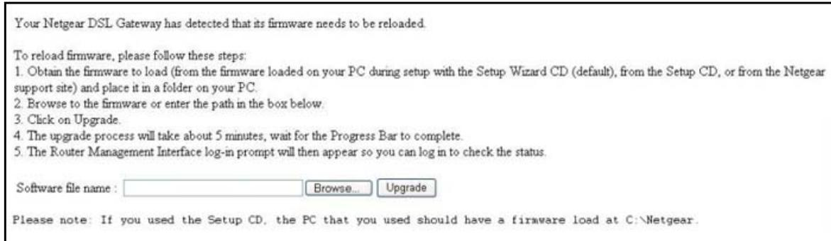
Figure 18. Reload firmware
