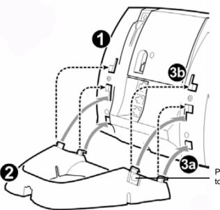
Press tabs on both sides to release and detach unit.
