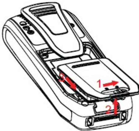
**Figure 14: Easy Replaceable Battery - Unlock the Lid and Remove the Battery**
