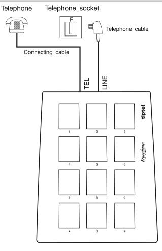
This is on the assumption that the telephone's connections are a normal pair of telephone cable connections. This is the case if the telephone complies with regulations TBR21 or ETSI ES 203 021. In the event that the "earth" and "alarm" contacts are used on your telephone socket, you must only use a two-core telephone cable.
