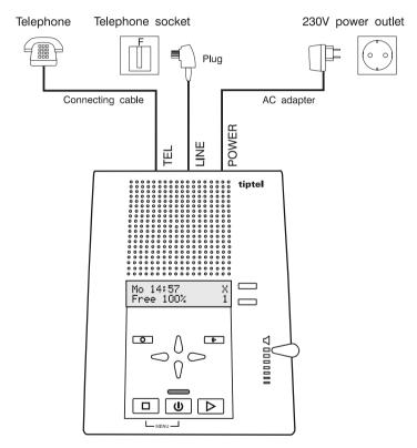
This connection option is recommended on the assumption that the telephone's connections are a normal pair of telephone cable connections. This is the case if the telephone complies with Regulations TBR21 or ETSI ES 203 021. In the event that the "earth" and "alarm" contacts are used on your telephone socket, you must exclusively use a two-core telephone cable.
