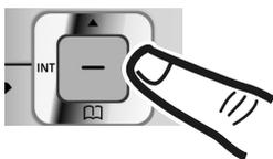
Press the **right** or **left** control key to change the input position and correct an entry.
