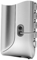
After removing the plastic cover, you can connect a headset to the left-hand side of your telephone with the 2.5 mm jack connector.
