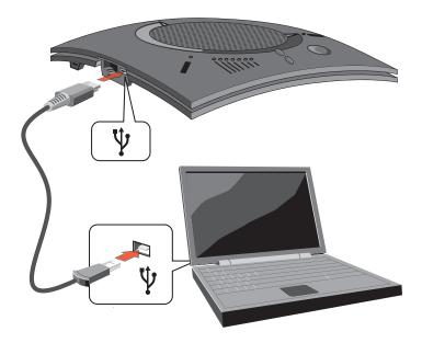
Once successfully connected to your computer, the CHAT 160 will automatically become the default audio device for Windows (speaker and microphone). When you run Skype, the CHAT 160 will also become the default speaker and microphone for Skype calls, replacing your computer's speakers and microphone. For more detailed information about using Skype and changing the audio settings, please refer to the Skype website at www.skype.com.
