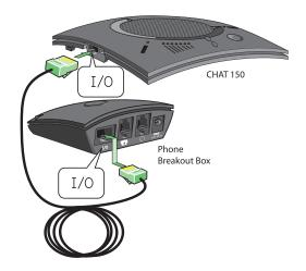
2. Using the included 2' RJ-9 telephone cable, connect the Phone Breakout Box's phone jack to your telephone's headset jack
