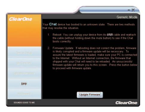
Use the following procedure to recover from interrupted firmware updates and unexpected programming errors:
