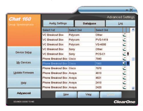
To view the settings for a particular device, select the device and click the **View** button, or double-click the device name. The **View Database Record** dialog appears.
