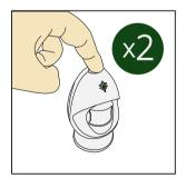
**4.** Double tap the energyEGG button to connect it to the Smart Light Switch
