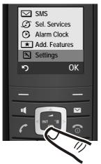
▶ Press the bottom of the control key until <a> Settings</a> is highlighted by the bar.
