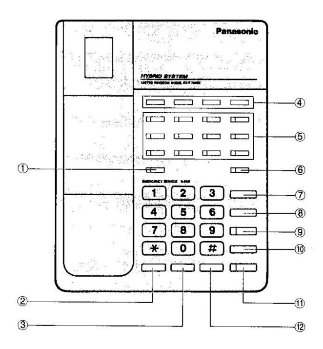
The KX-T7050E is designed especially for the visually handicapped operators: TRANSFER button, SP-PHONE button, and dial key "5" of KX-T7050E have a raised pip to aid them to locate the buttons and keys.
