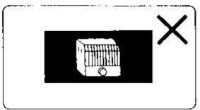
The unit should be kept free of dust, moisture and vibration, and should not be exposed to direct sunlight.
