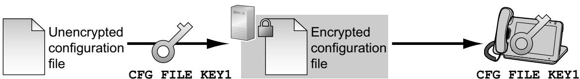
To use this method, an encryption key is required to encrypt and decrypt the configuration files. A preset encryption key unique to each unit, an encryption key set by your phone system dealer, etc., is used for the encryption. When the unit downloads an encrypted configuration file, it will decrypt the file using the same encryption key, and then configure the settings automatically.
