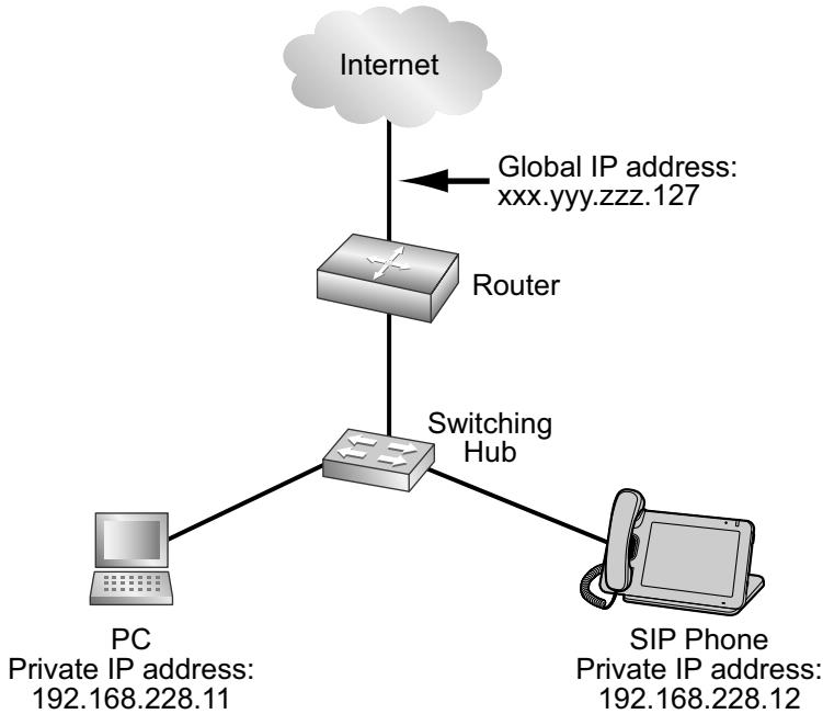
If the unit is connected to a network that uses a NAT router and a private IP address is assigned to each terminal on the network, depending on your phone system's setup, you might need to configure the unit and router so as to use NAT Traversal techniques.
