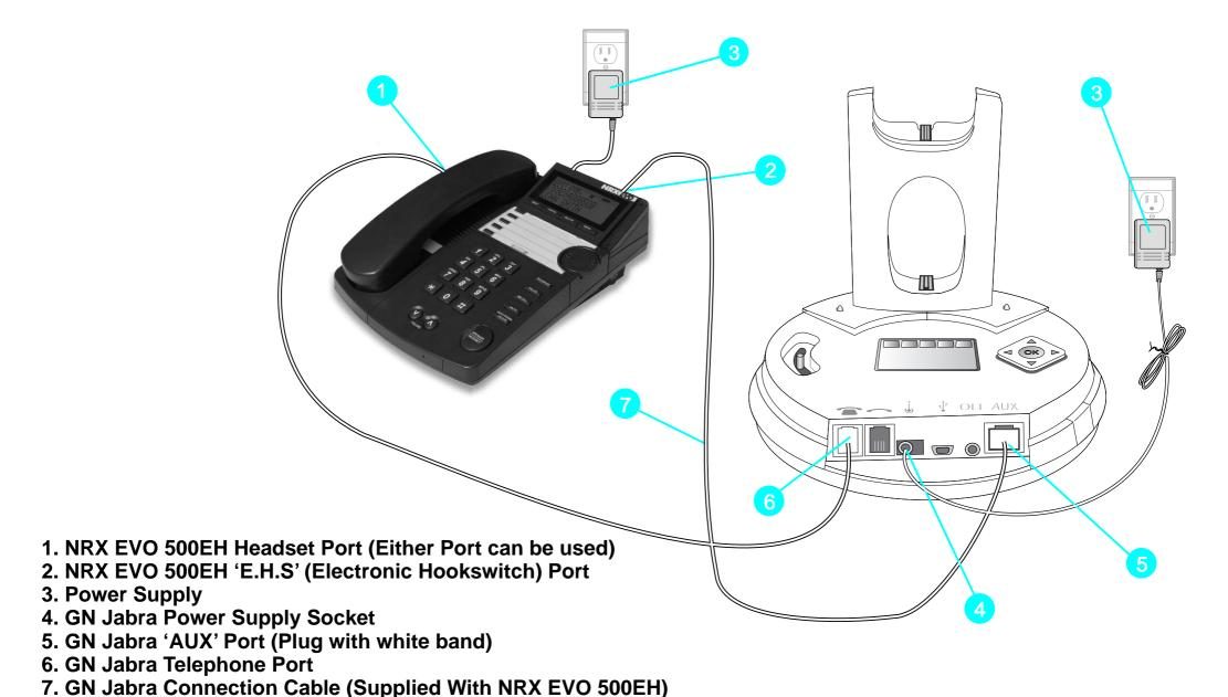
NOTE: The NRX EVO 500EH replicates the functionality of the GN1000 RHL Handset lifter so the Headset base needs to be set to the 'GN RHL' setting. Please refer to your headset manual for information on how to do this.
