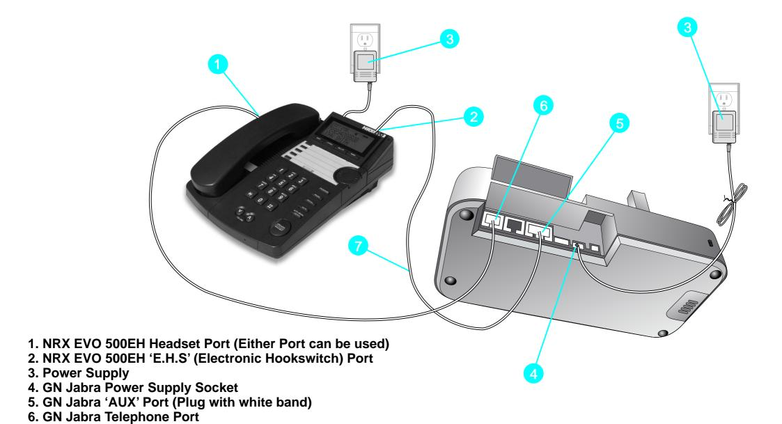
NOTE: The NRX EVO 500EH replicates the functionality of the GN1000 RHL Handset lifter so during the initial Headset base setup, select the 'GN1000' option <u>not</u> the 'Electronic Hookswitch' setting.
