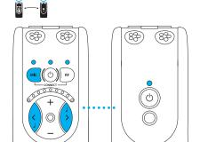
The sound from the Transmitter Unit is mixed with the sound from the internal microphone. You can adjust the balance between the Receiver Unit and the Transmitter Unit's microphone by holding down the M button(5) at the same time as setting the balance using the < (11) or > buttons (12).
