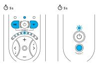
A "running light" on the Receiver Unit's Volume and Tone LED Indicator (8) moving towards the centre indicates that the link has been established.
