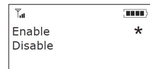
» Note: When enabled, Auto Disconnect will automatically hang up the phone once the other end is disconnected.
