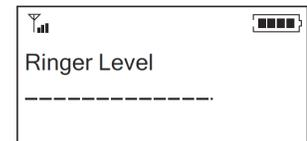
» Note: Ringer volume is indicated by a horizontal bar on the LCD screen.
