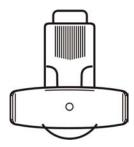
Belt clip and adapter for the telephone. The adapter is clipped onto the telephone.
