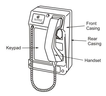
Commander is a family of rugged, weather-resistant telephones manufactured from moulded glass-reinforced polyester. A range of handset types and keypad configurations are available.
