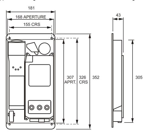
To flush-mount the telephone to a wall:
