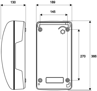
1. Using a suitable tool, punch out the 4 holes in the rear enclosure, taking care not to damage or dislodge the plastic bushes. Only four of the eight holes are required - the outer ones are recommended. The inner holes are provided to be compatible with older-style mounting posts, and should be left intact if not used. If the inner holes are used they must be fitted with the supplied plastic bushes.
