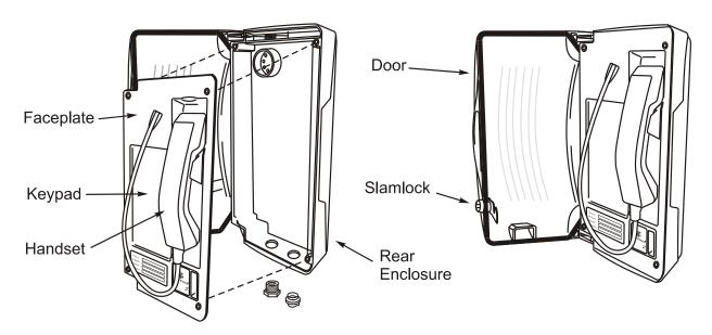
Titan is a family of rugged, weather-resistant metal-bodied telephones available with a range of handset types, keypad configurations, colours and enclosures, based around a common faceplate style.
