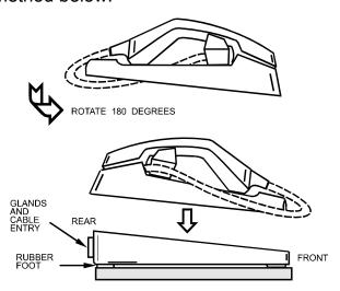
To provide a 'rake' for convenient operation, the Front Casing may be turned through 180° before it is fitted to the Rear Casing. Thus the cable entries are at the rear of the telephone.
