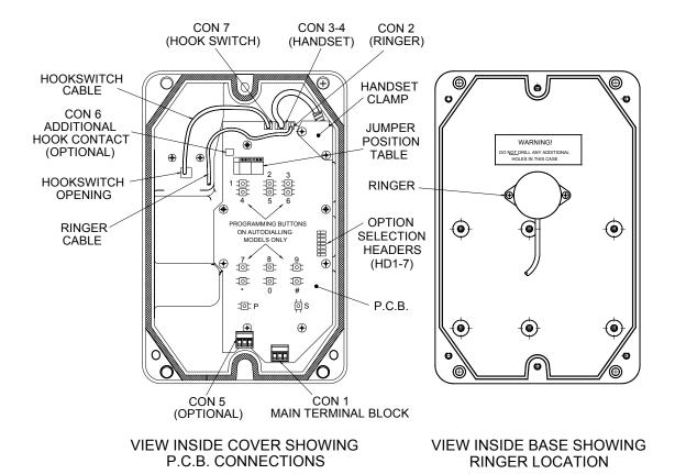
2. To prepare for installation, undo the three retaining screws shown to remove the front casing from the rear. The screws are captive in the
