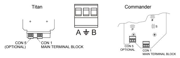
The centre earth terminal is intended as an optional connection to a local earth for the purpose of enhanced protection from lightning transients, and is not required in terms of user safety from the telephone network.
