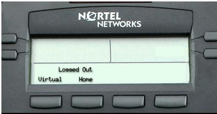
When activated for Virtual Office by a remote telephone, your office telephone is *logged out* and no longer operational.
