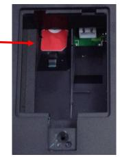
Connect the battery pack into its connector and position in place
