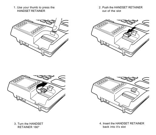
Figure 2 Handset Retainer for Wall Mounting
