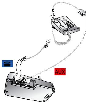
Figure 13.1: Connecting using an electronic-hookswitch adapter (Jabra LINK series)
