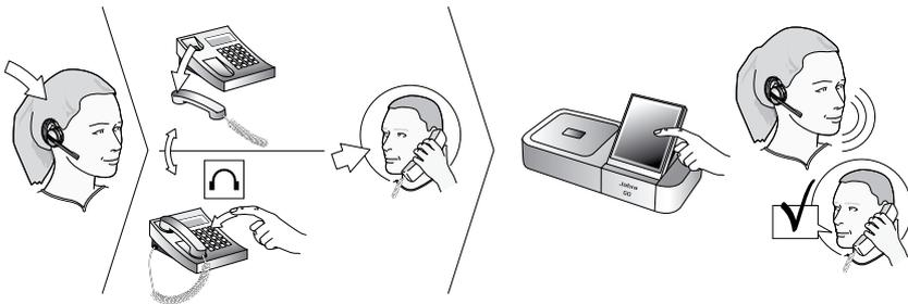
Figure 12: Setting the microphone level manually
