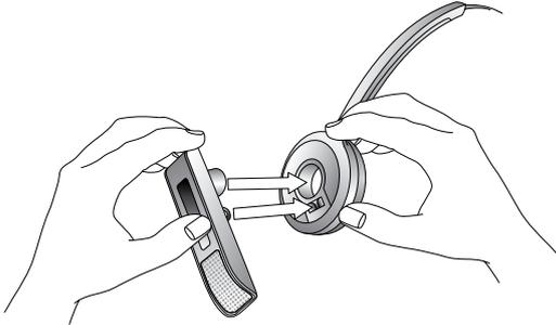
Figure 26: Attaching the Jabra GO headset to a head- or neckband
