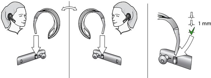
Figure 25: Attaching the ear hook
