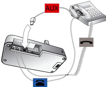
Figure 13: Connecting to a GN1000 Remote Handset Lifter
