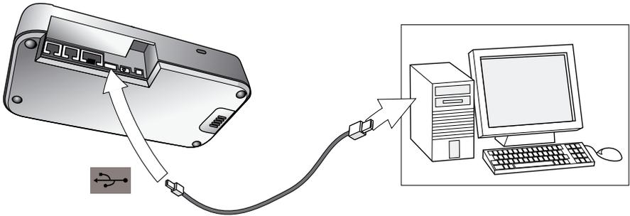
Figure 14: Connecting to a computer
