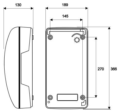
Using a suitable tool, punch out the 4 holes in the rear enclosure, taking care not to damage or dislodge the plastic bushes. Only four of the eight holes are required - the outer ones are recommended. The inner holes are provided to be compatible with older-style mounting posts, and should be left intact if not used. If the inner holes are used they must be fitted with the supplied plastic bushes.
