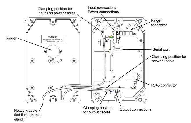
Take particular note of the cable clamping arrangements – all cables must be securely clamped in the clamps provided.
