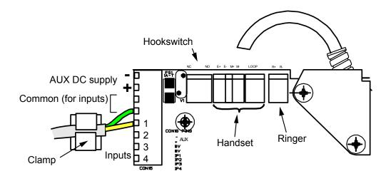
External power supply – 24-48Vdc, 200mA
