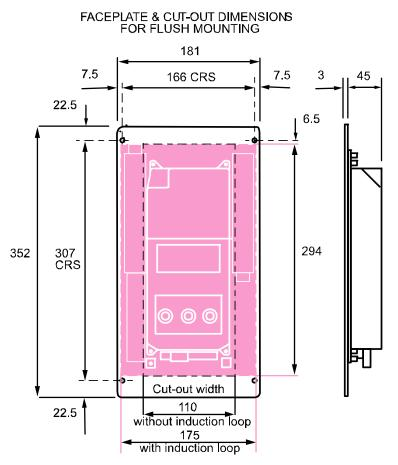
To flush-mount the telephone to a wall:
