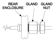
**IMPORTANT**: If only one gland entry is used, the blanking plug fitted to the second gland position must be left in place.
