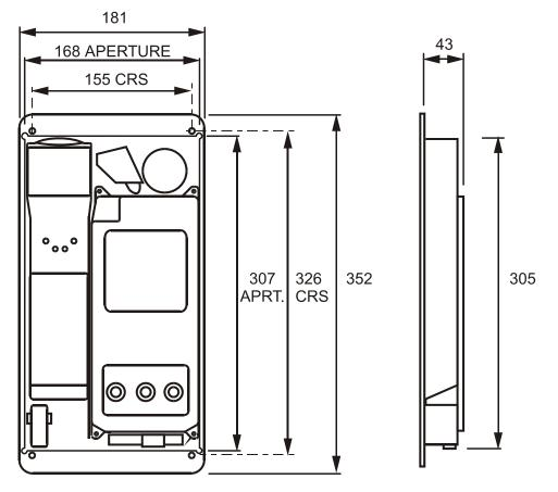
To flush-mount the telephone to a wall:
